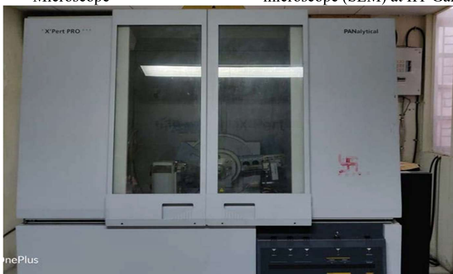
c) X-ray diffraction (XRD) on a Pan Analytical X'pert Pro system at MSU, Baroda.
