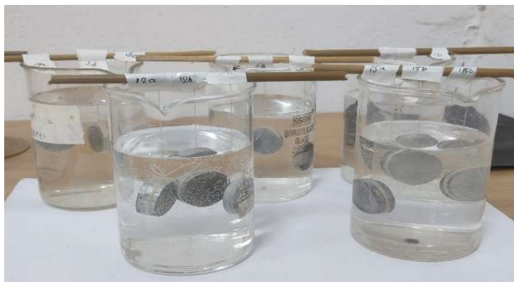
Figure 3.11 Experimental set up for standard weight loss method.
