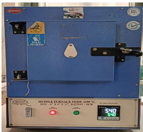
Figure 3.7 Muffle furnace at Dr. S & S. S. Ghandhy College of Engineering & Technology, Surat.
