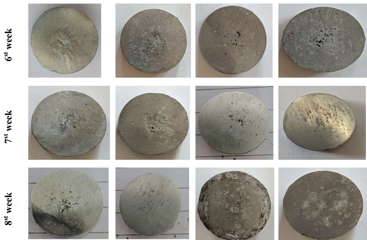
Figure 4.17 Surface morphologies of Al-6.5Mg-xSi alloys in the heat treated condition after weekly exposure to the corrosive medium.
