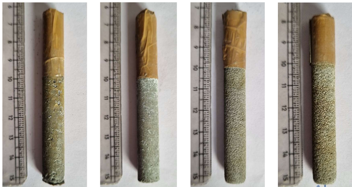
Figure 4.24 Surface morphology of Al-6.5Mg-xSi sacrificial anode specimens after Anode performance measurement in both as-cast and T6 heat treated conditions.
