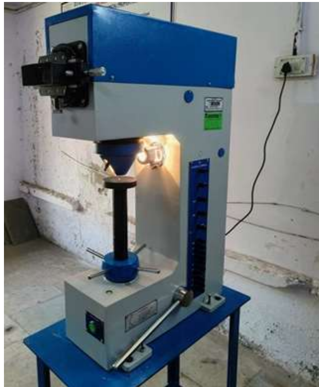
Figure 3.9 Brinell Hardness tester at Dr.S &S.S.Gandhy College of Engg. & Tech., Surat.
