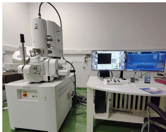
b) JEOL JSM 7900F scanning electron microscope (SEM) at IIT Gandhinagar
