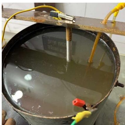
Figure 3.13 Experimental set up: MS vessel fills with electrolyte and specimen.
