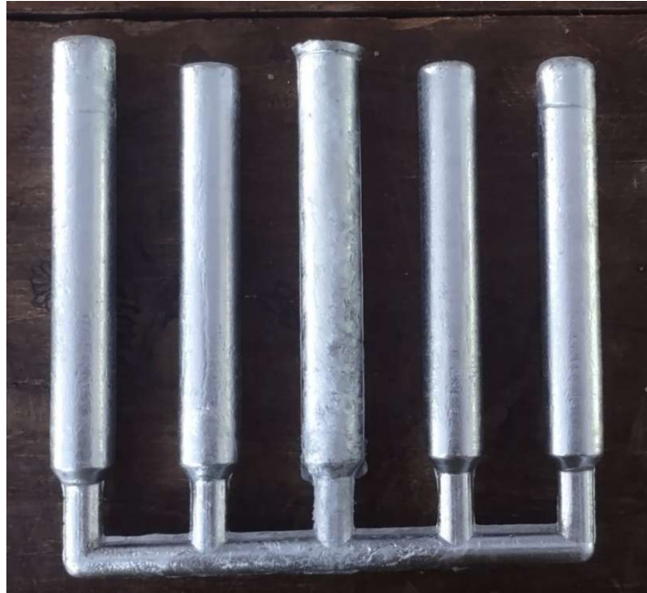
Figure 3.4 Die Cast Al-Mg-Si Alloy.
