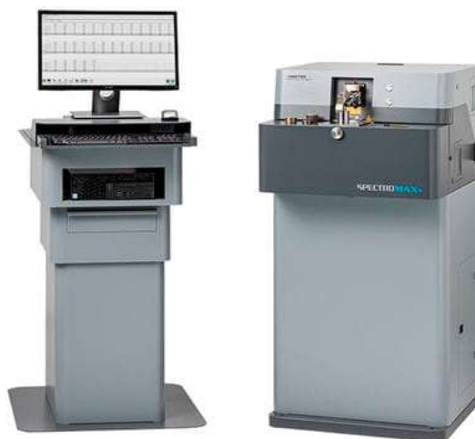
Figure 3.8 Optical Emission Spectroscopy.
